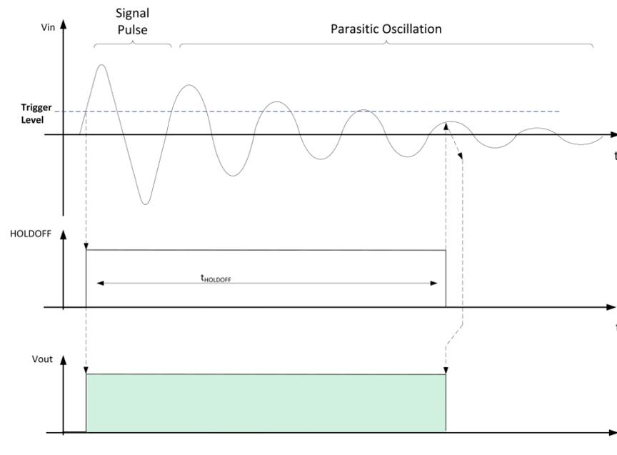
The holdoff function is a powerful feature to suppress parasitic triggering. To get further information about it, please see “TN608-02 Blocking parasitic triggering with the HOLDOFF function”.
