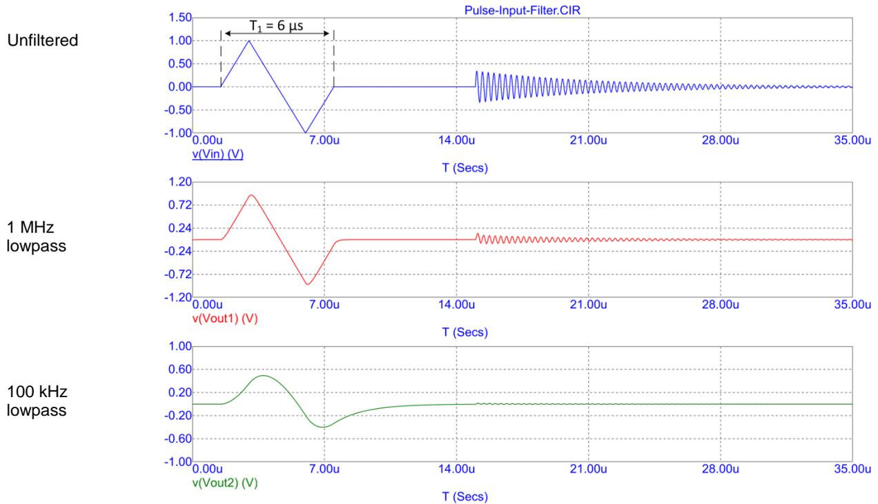
PI608 Versatile Trigger Unit has a maximum bandwidth limit of 1MHz. In general that’s a good setting for most industrial applications. RF rejection is provided, while the sensor signal remains unaffected.
