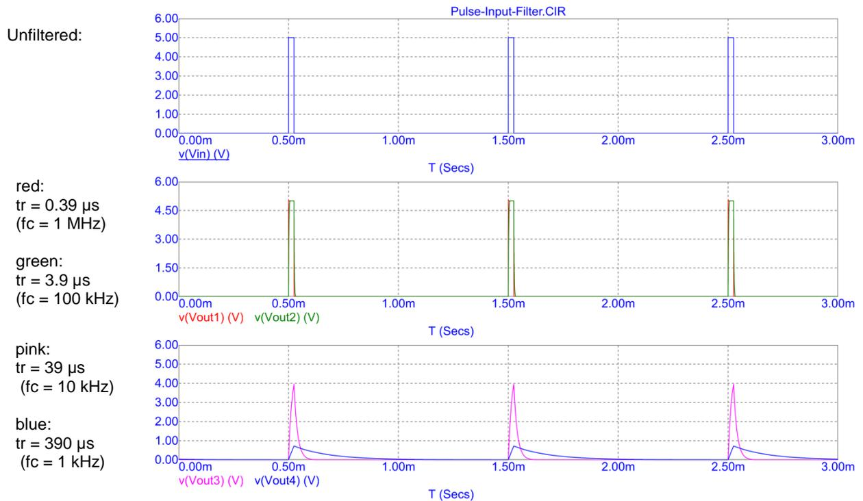
It is easy to see that a filter with a rise time longer than the pulse width will change the shape of the pulse dramatically. The pulse becomes flat and delayed. Proper triggering may become impossible.
