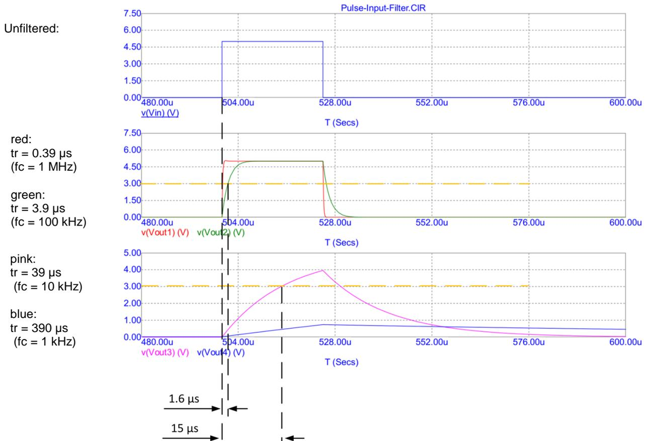
As we can see a filter with a rise time of 3.9  $\mu$ s (100 kHz) makes a delay of 1.6  $\mu$ s. That can be already quite a lot for a 25  $\mu$ s pulse.
